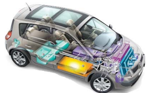
The Renault Scenic prototype fuel cell vehicle will incorporate Nuvera's STAR gasoline fuel processing technology.
